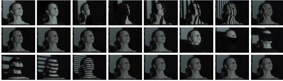
Fig. 2. 24 binary structured light patterns for a given frame
