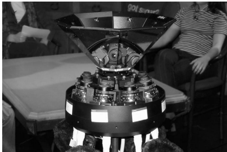
Figure 7. 360-degree camera system with eight facets, each capturing a 45 degree arc of the surrounding space.
