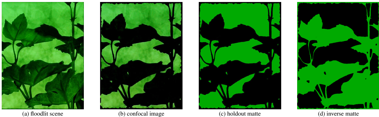
Figure 8: Synthetic aperture confocal imaging. (a) shows a plant in front of a diffuse white screen. Coded aperture imaging was used, with 32 trials of sinuous patterns. However, to reduce chromatic aberration only the green channel was used. Since the focal plane coincided with the screen, only it remains bright in the confocal image; the plant is nearly black. Dividing (b) by (a) to eliminate shadows, then contrast-stretching the result, produces a holdout matte (c) and its inverse (d). These mattes are used in figures 10(b) and (c).
