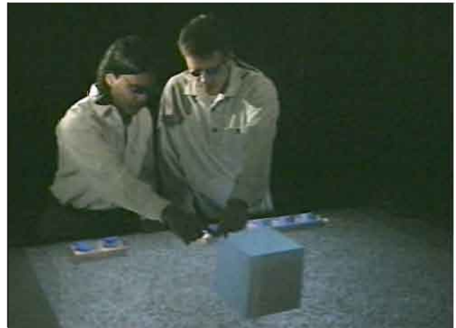
Figure 1: Two users simultaneously view a shared virtual environment on the Responsive Workbench. Calibration ensures that when they point to the same feature on the virtual cube, their fingers touch. Note that the image on the Workbench is rendered for the point of view of the camera.
