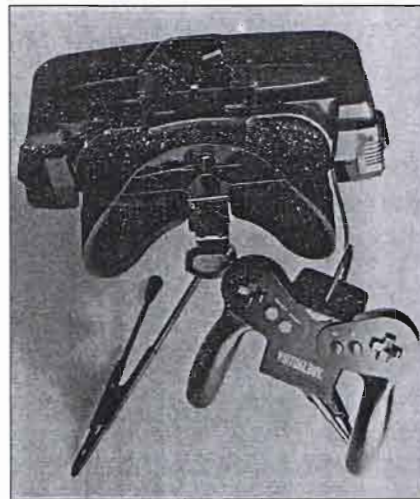
Figure 2. Virtual Boy fixed stereo display. (Courtesy of Nintendo)
